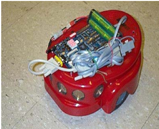
Amigobot controlled by NIOS SOC board. Extra FPGA logic was used for serial ports, sensor interfaces, and an LCD interface.
