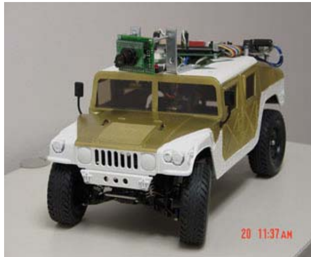
R/C Hummer with NIOS SOC board and CMUCAM. Extra FPGA logic was used for servo PWM controllers.
